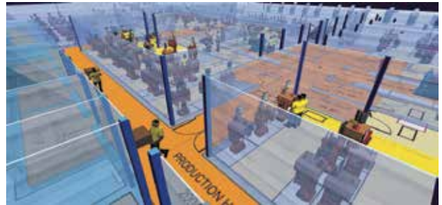
Figure 2: DES models help characterize uncertainty and variability inherent to the operations, while helping visually communicate the results. (Source: CRB.)
